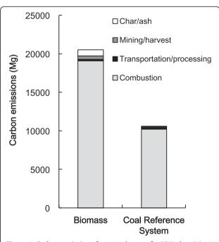
Figure 3 Carbon emissions for 8000 hours of 5 MW electricity produced from bioenergy and a coal reference system.
