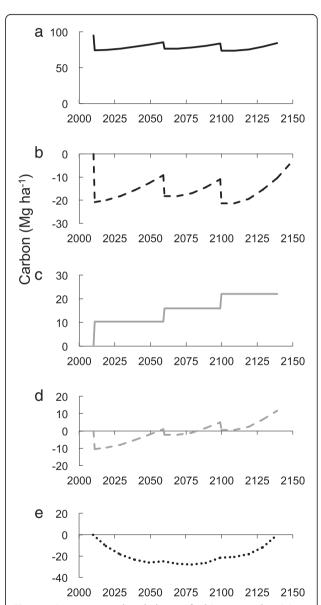
**Figure 4** Long-term carbon balance of a bioenergy electricity production. (a) Total stand carbon (b) net stand carbon (c) cumulative carbon offset through bioenergy production and avoided coal emissions and (d) net stand carbon including carbon offset in a stand with repeated treatments. (e) Forest wide carbon balance with forest treatments to fuel bioenergy bioenergy production every year through 2100.
