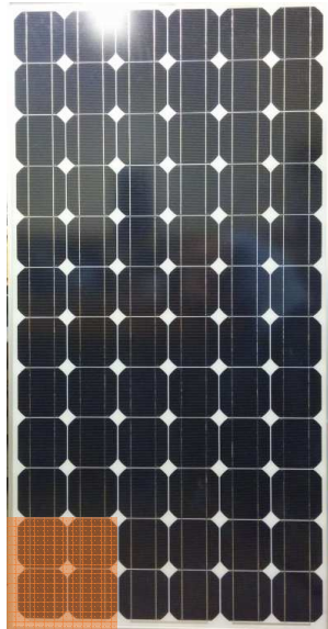
Figure 5.10: Shading pattern for the partial shaded substring.
