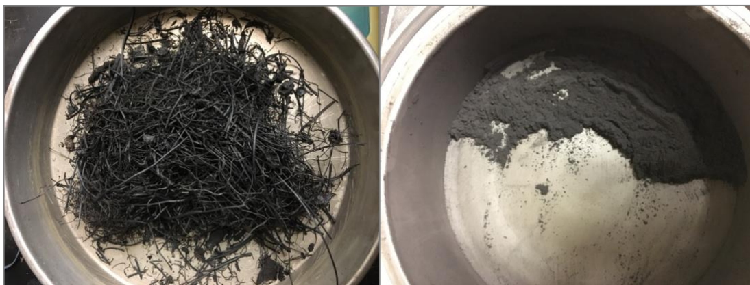
Figure 2-3: Burned litter before (left) and after (right) mechanical homogenization for 15 seconds.
