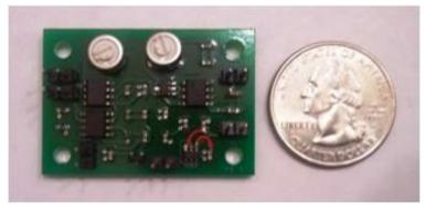
(a) Modular single EEG channel amplification and filtering circuit board.
