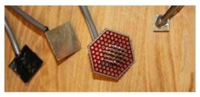
(b) Three types of dry EEG electrodes used: (Left to Right) flat-type, pin-type, and clip-type.
