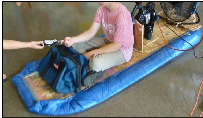
Figure 13: Using a spring scale to measure friction
