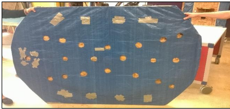
Figure 14: Skirt holes patched with duct tape
