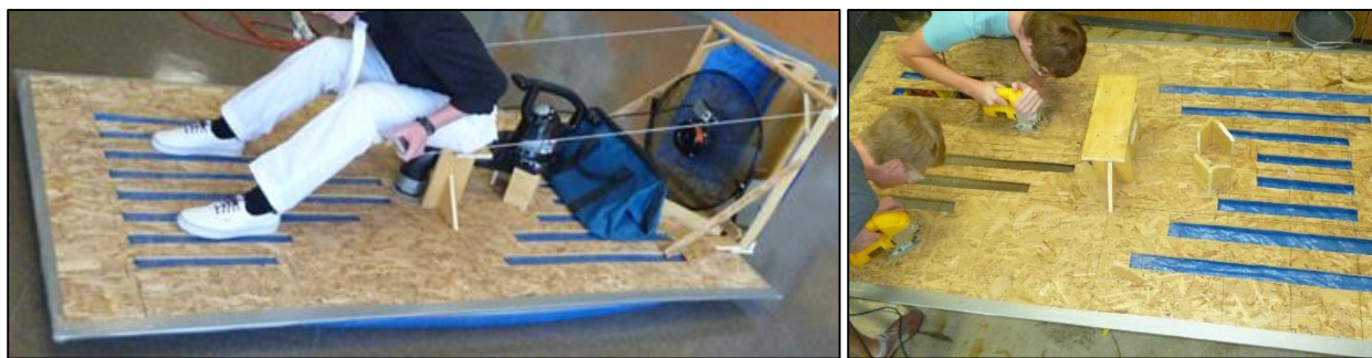
Figure 18 (left): Rick’s hovercraft undergoing performance testing
